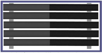
Image 7.3. Diagram of a tire tread fence
