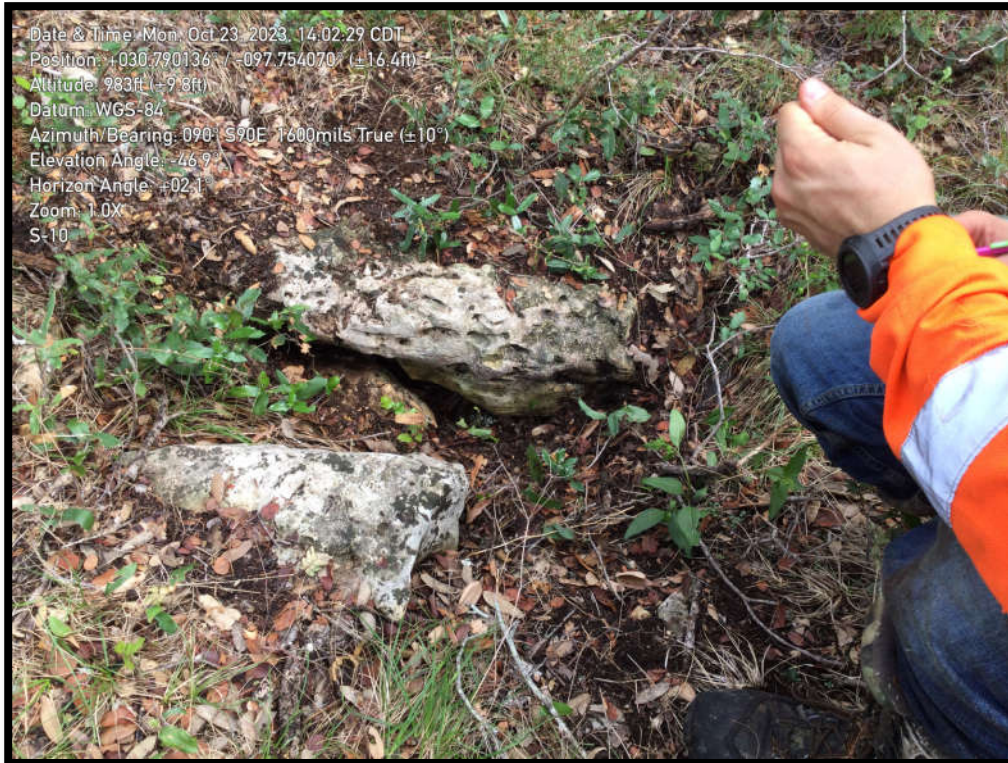
S-10: Solution cavity located on the heavily vegetated central part of the Site.
